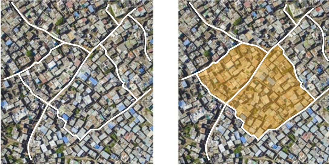
Figure F.9: Hypothetical example of the superblock layout approach - desire lines (L) creating large land parcels (R)
