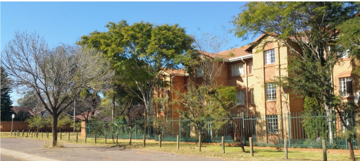
Figure H.17: See-through fences and street-facing buildings allow for visual contact between buildings and the street
