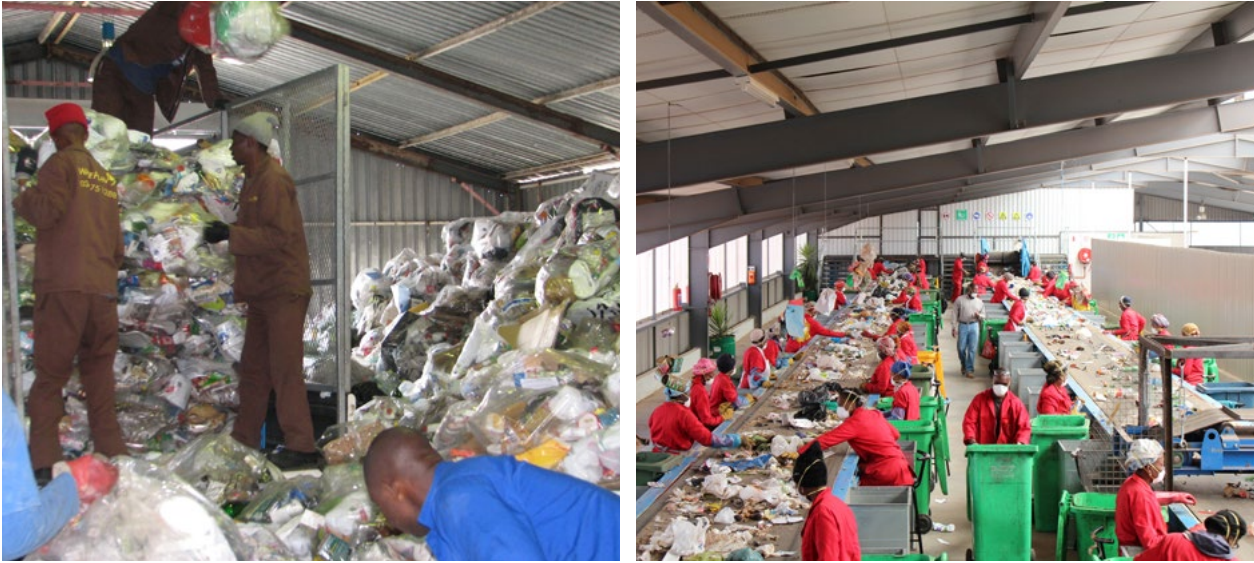
Figure M.10: Recyclables offloaded at a clean MRF (L) and sorting tables at a dirty MRF (R)
