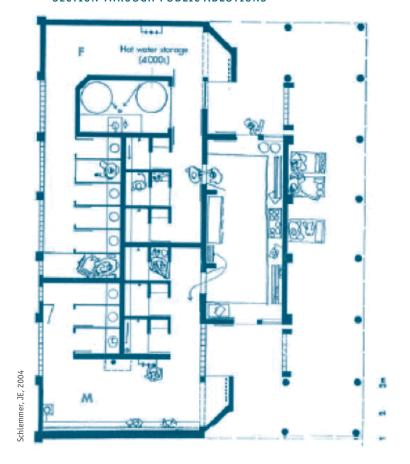
A section and plan of the public ablution facilities. Solar panels fitted to the roof provide cheap harvesting of power, used to warm the water used.
