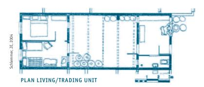
Plan of the living and trading unit with the storage area used as a private dwelling space for the unit's residents. The structure overhead is made of bluegum poles with a removable tarpaulin cloth to regulate solar gain.
