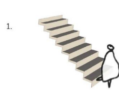
1. Galvanised steel single staircase to first floor
