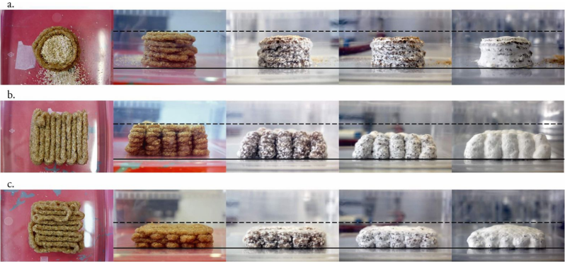
The growth process of various extrusion patterns (Elsacker, Peeters & De Laet 2022)
