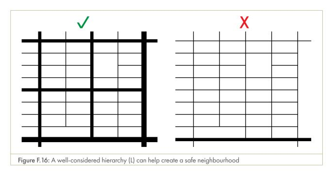
A hierarchy of streets could assist in reducing conflict between through-traffic and local access-seeking traffic. Local conditions should guide the hierarchy, and care should be taken to consider all users of the streets, not only vehicle users. The separation of different types of traffic and road users may also not always be appropriate, and therefore a rigid hierarchy is not advisable. The following should be considered when preparing a hierarchical street layout:
