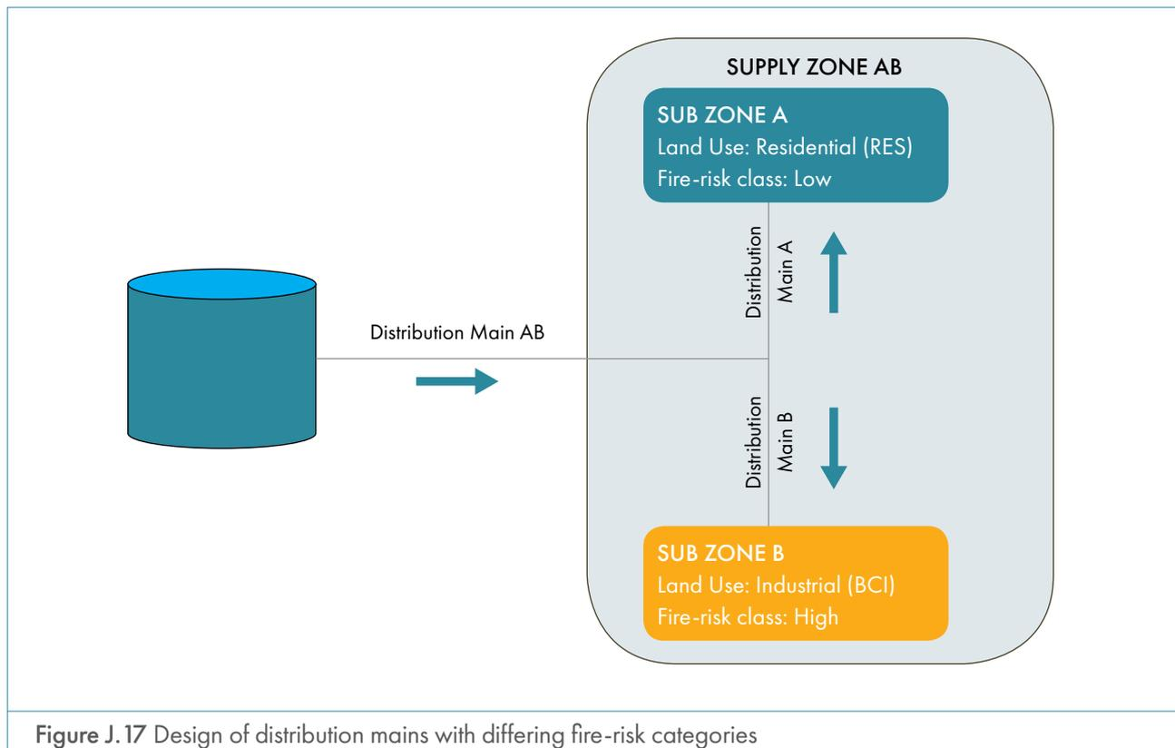
Figure J.17 Design of distribution mains with differing fire-risk categories
