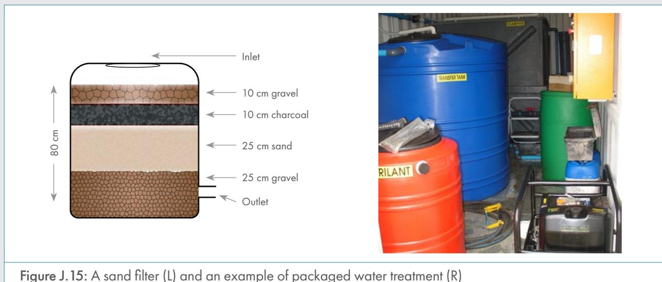
Figure J.15: A sand filter (L) and an example of packaged water treatment (R)
