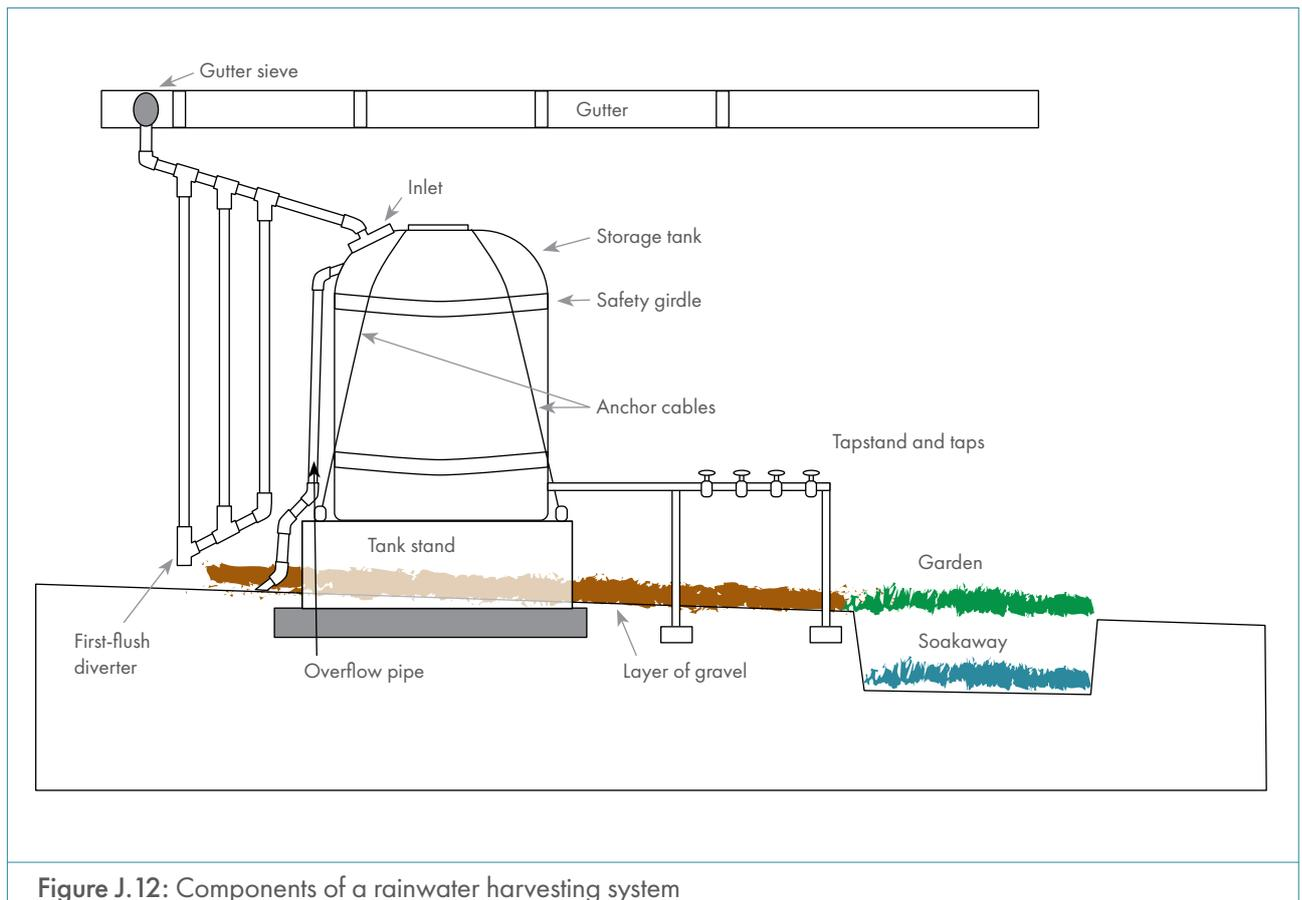
**Figure J.12:** Components of a rainwater harvesting system
