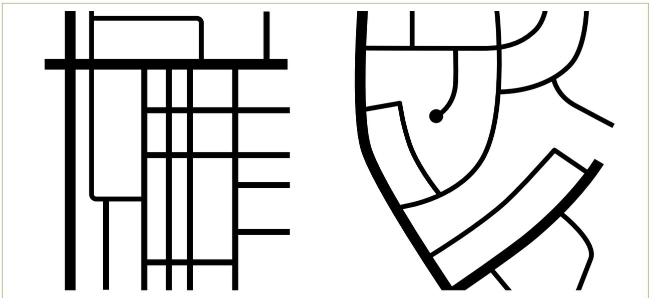
Figure F.5: The fragmented parallel grid street layout (L) and the warped parallel grid street layout (R)
