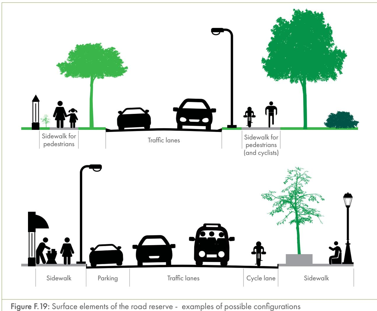
Figure F.19: Surface elements of the road reserve - examples of possible configurations
