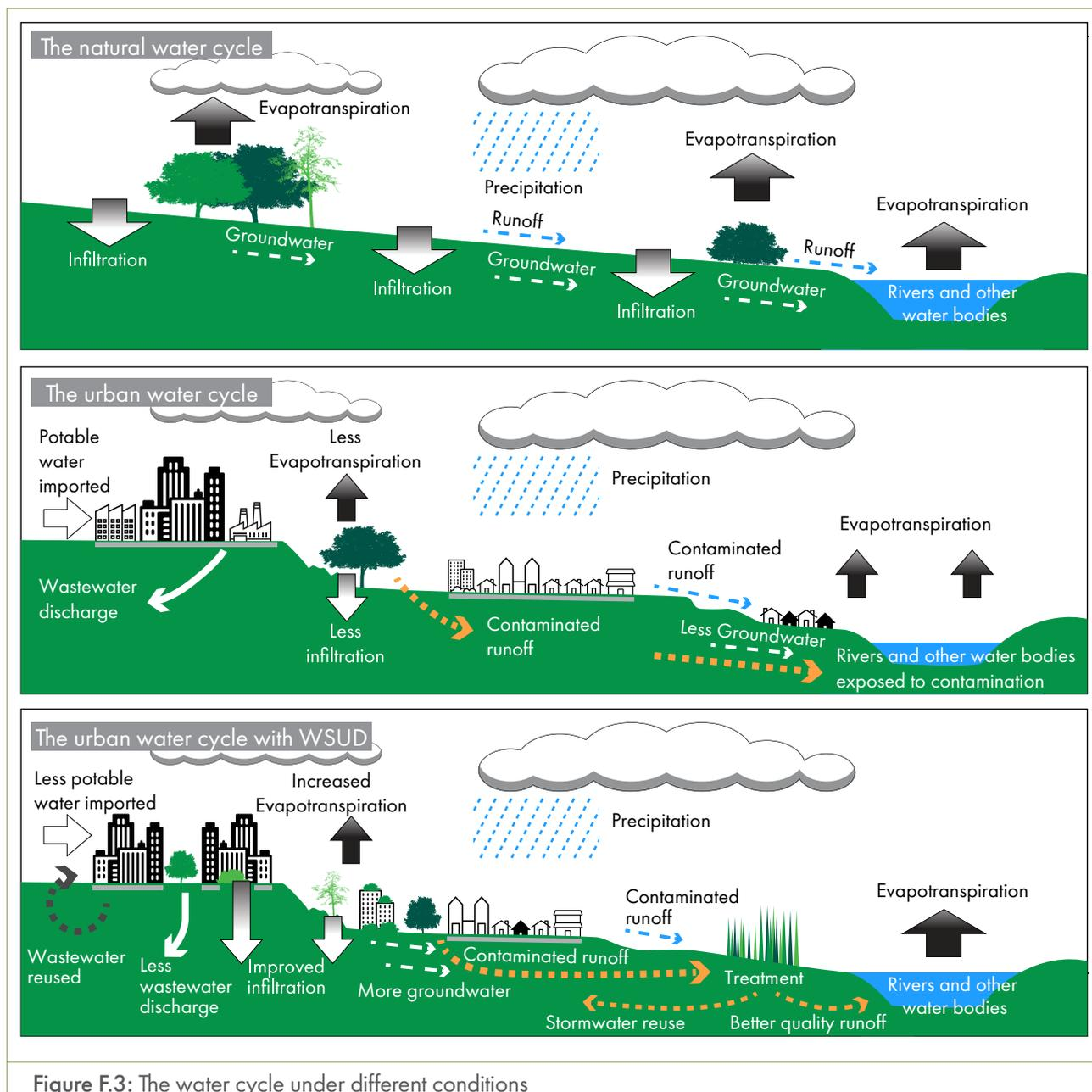
Figure F.3: The water cycle under different conditions
