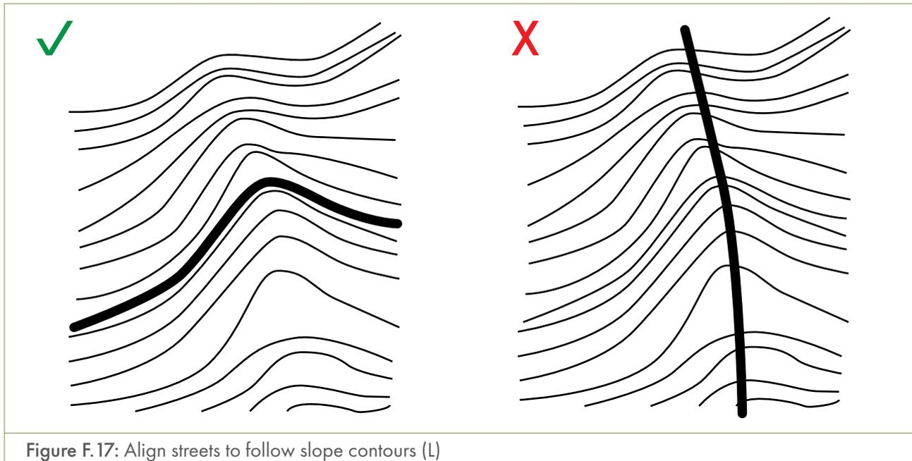
Figure F.17: Align streets to follow slope contours (L)
