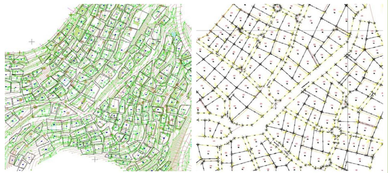
Figure F.10: Example of the bottom-up de facto layout approach
