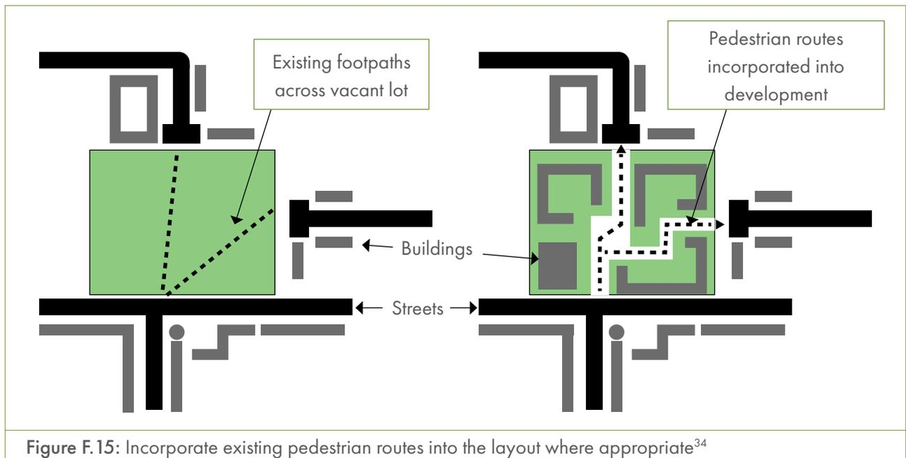
Figure F.15: Incorporate existing pedestrian routes into the layout where appropriate<sup>34</sup>
