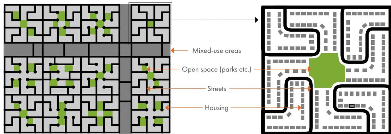
Figure F.7: The fused-grid street layout
