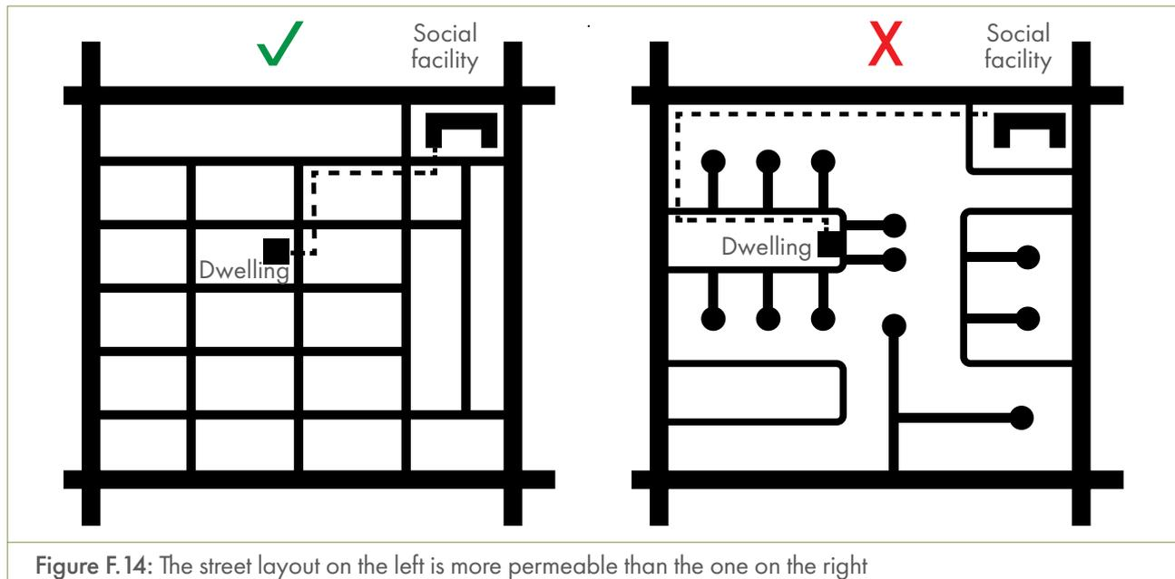
Figure F.14: The street layout on the left is more permeable than the one on the right
