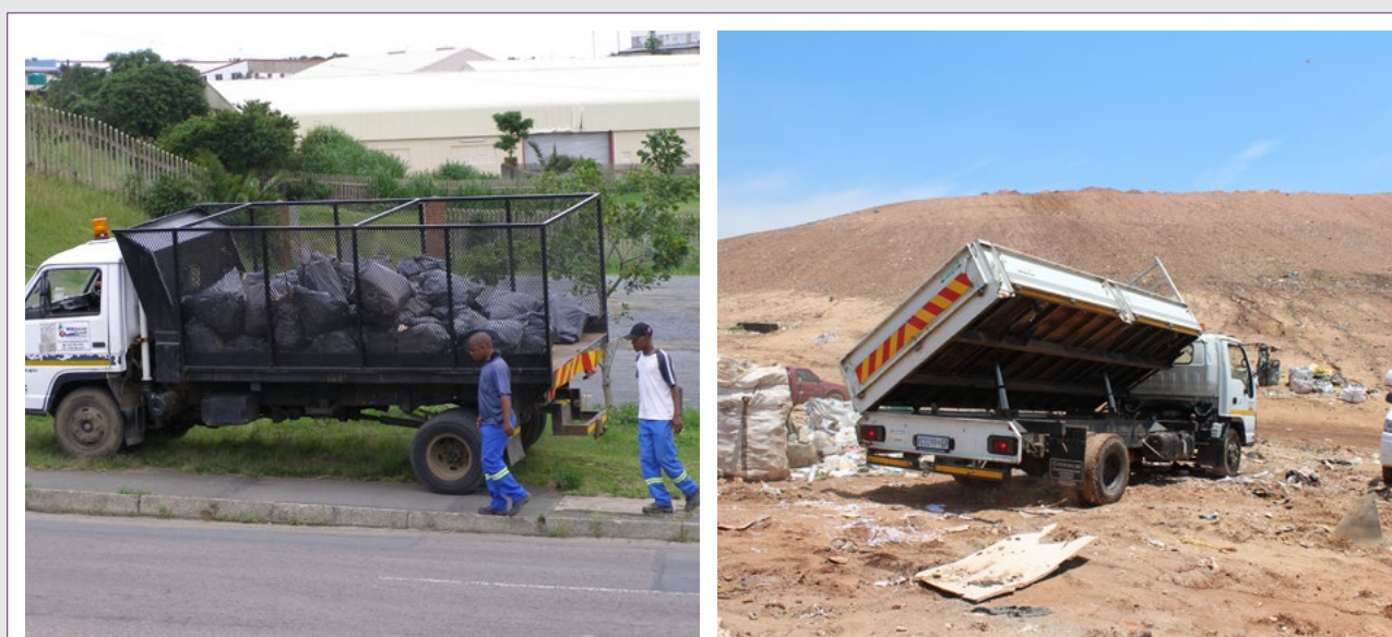
Figure M.7: Examples of a caged truck (L) and a tip truck (R) that are used for waste collection
