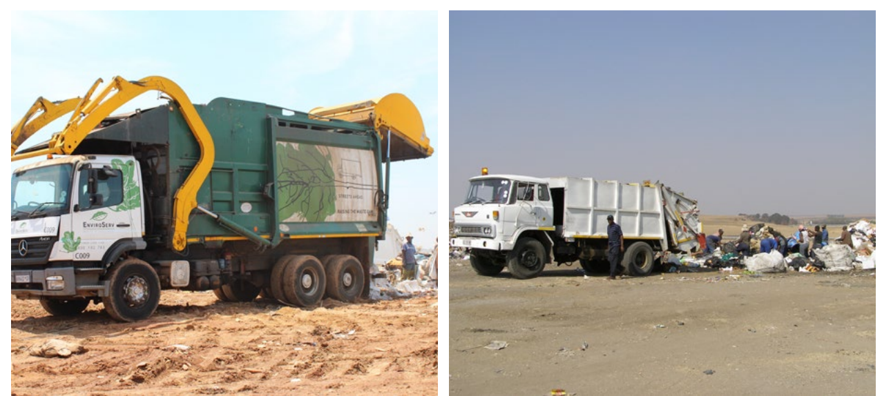
Figure M.8: Examples of a front-end loader (L) and a rear-end loader (R) that are used for waste collection
