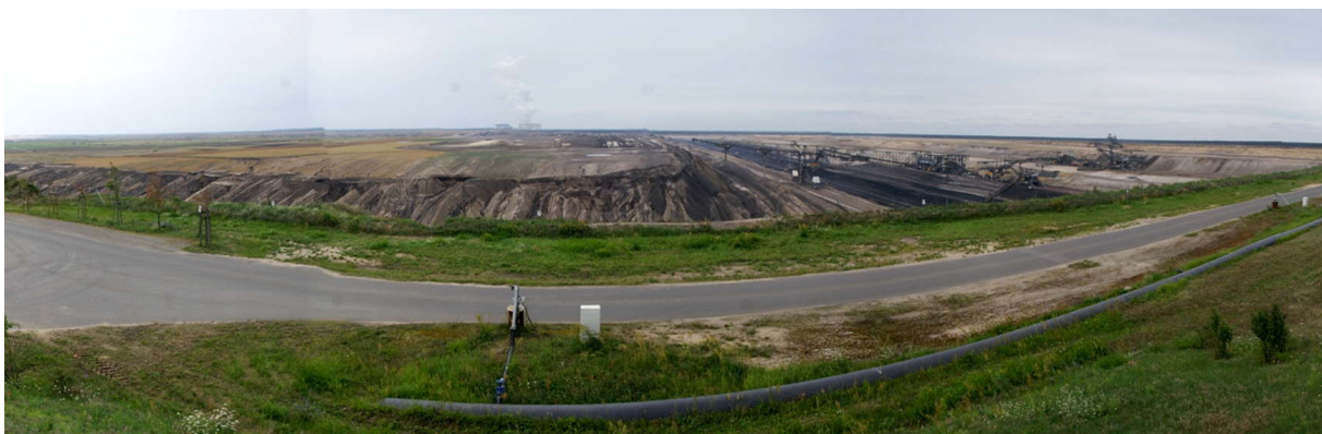
Fig 1. Brown coal surface mine Tagebau Jänschwalde in the German Cottbus Industrial District – a view from an observation terrace at a cycling track (photo by the author, 2013). The display of the site of the mine enables visitors to watch all the stages of mining works: coal extraction (in the middle), uncovering the deposit for extraction (on the right) and reclamation of the post-excitation sites (on the left).
